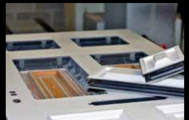
Door after routing operation
